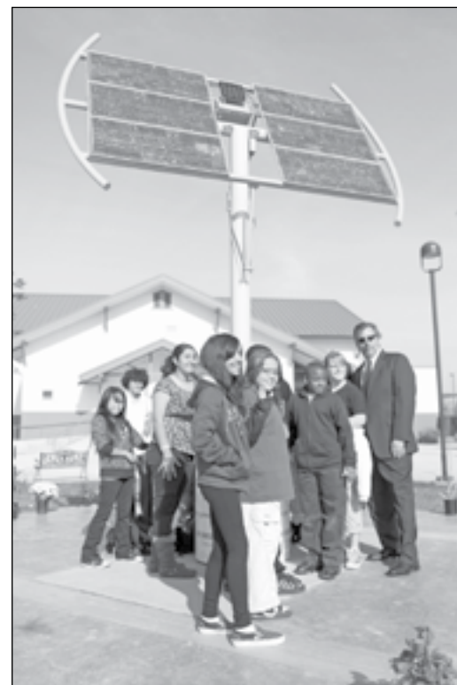
Photo courtesy Students of the School of Engineering and Science stand in front of the school's new Solar SunFlower, an 18-foot-high outdoor learning lab. Students can rotate the panels to see how much electricity the sun provides and study changes in the voltage and current being generated.
